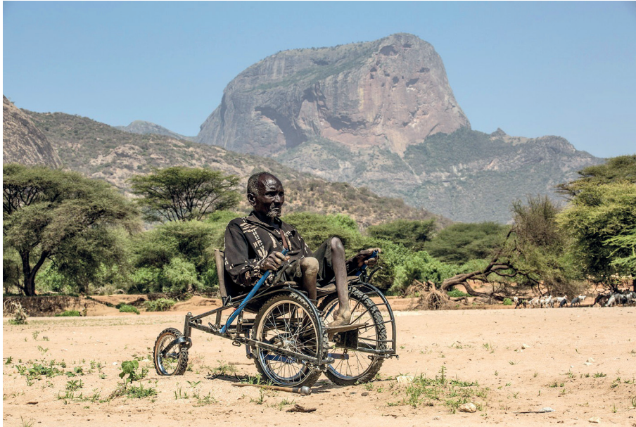
Figure 14: The SafariSeat first prototype (with lever propulsion)
